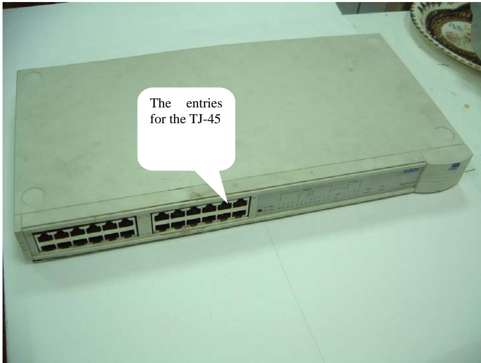
Fig. 12. Example of a Hub with 24 ports (3Com. SuperStack II ®) .
