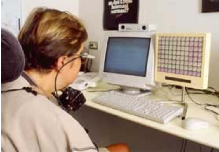
Fig. 4. Adaptive computer use: head pointing.. www.rtdhetdorp.nl
